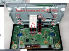
2 Remove 6 screws and FPC cables
